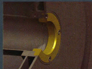
Arbor provided with interchangeable screwed bushings
