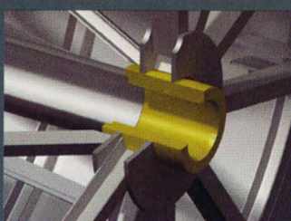
Arbor provided with machined bushings (mainly for internal process or for high-speed process)
