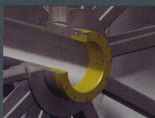
Arbor provided with interchangeable screwed bushings
